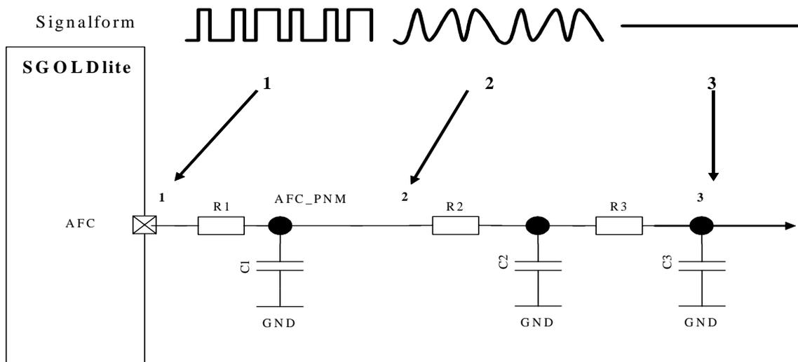
Waveform of the AFC signal from SGOLDlite to Oscillator
