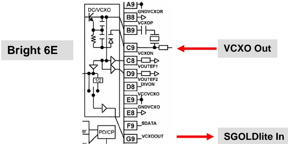
To compensate frequency drifts (e.g. caused by temperature) the oscillator frequency is controlled by the (RF\_AFC) signal, generated through the internal SGOLDlite (D1000 (Functional A9)) PLL. Reference for the "SGOLDlite -PLL" is the base station frequency received via the Frequency Correction Burst.
