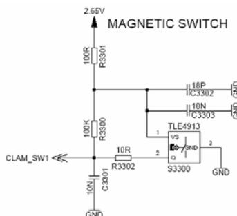
A magnet is placed inside the lift housing. The magnetic switch **S3000** is used to identify the position of the housing. The output of the switch is connect to the **SGOLDLITE** (Serial interface C20)
